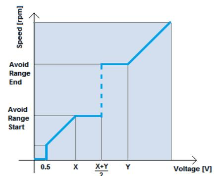
**i** This function should be avoided when used in close control loops application or unstable conditions of the fan could occur.
