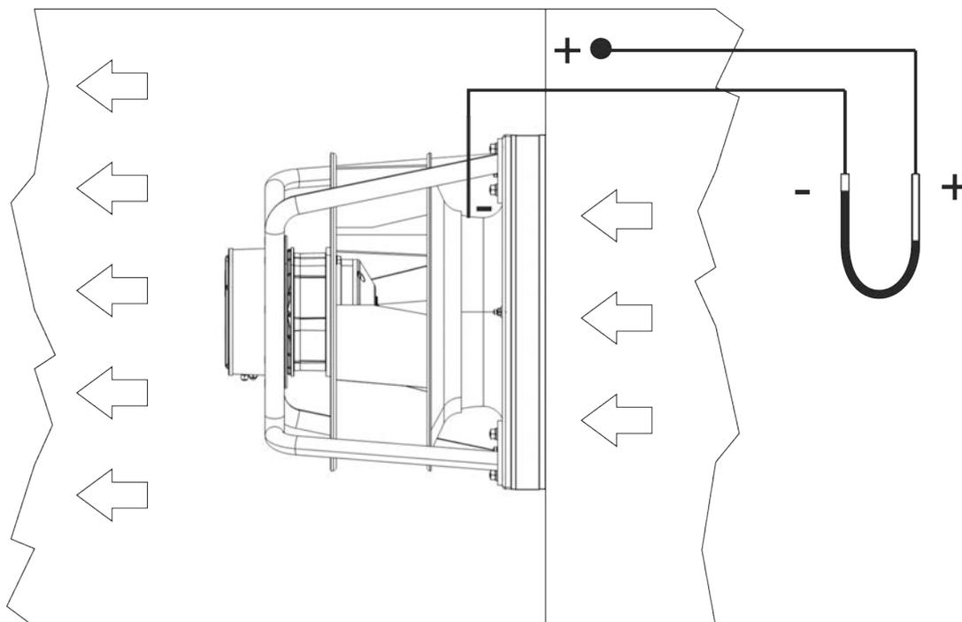
The Volumeter device is based on the Venturi principle, sensing the suction which is produced, in the throat section of the fan inlet nozzle or bell-mouth, by the airflow entering the fan.
