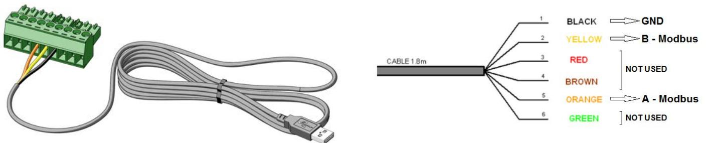
To connect OFFLINE the driver to a PC when the fan is powered off, a USB to UART converter can be used: K431A6 for 1-phase drivers and K431F7 for 3-phase drivers.
