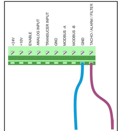
The same analogue output channel can be reconfigured, by changing the value in Holding Register 46 (see paragraph 18.3 at page 41), as a Digital Alarm Output (refer to chapter 19 and paragraph 19.4), or in one of the alternative alarm modes described in paragraphs 12.1 and 12.2.
