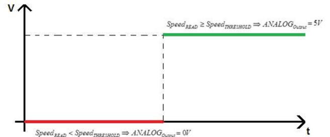
To activate this feature, the **Holding Register 46** must be set at value 2 and the required Speed Threshold value must be set into the **Holding Register 55**. The digital output of the driver changes its status (see above figure).
