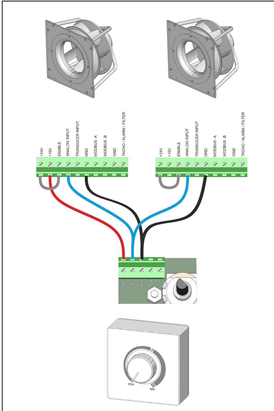
If an ext. 4-20mA device is used, it is necessary to add 0.1% precision resistances between the ANALOG INPUT and GND.
