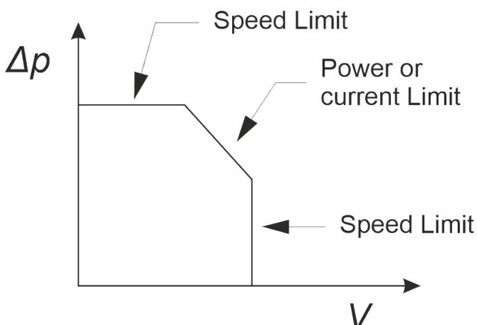
The drivers are protected against overload conditions and a safe operating area is defined by a limit of speed, output power and motor current.
