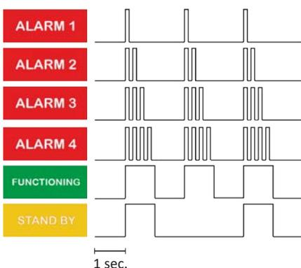
The system status can be displayed through the LED on the driver plate (see par. 9.6). In the following figure on the right the blinking LED is shown.
